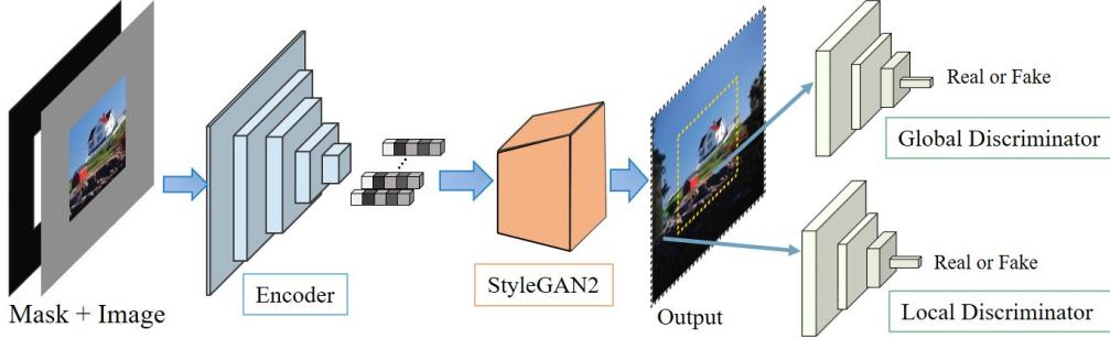
Fig. 4. Overview of image extrapolation architecture. The conditional encoder first embeds a masked image to a latent code in StyleGAN2’s latent domain. StyleGAN2 then recovers the partial images and generates diverse samples in the extrapolated region. The global discriminator takes the entire image as input, while the local discriminator takes the extrapolated region as input. Both discriminators are trained to distinguish between the real and generated images.
