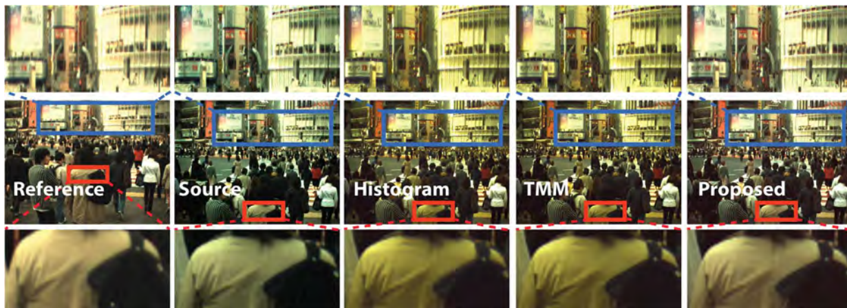
Fig. 4. Color corrected result of the Crowd sequence (60th frame). Source: input view that color correction need to be performed; Histogram: result with [3]; TMM: result with [4]; Proposed: result with our method.
