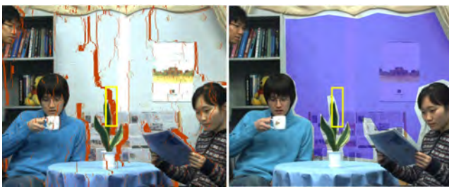
Fig. 8 Depth aware candidate search for patch-based inpainting, with which reference patches of the disoccluded areas (see the yellow rectangle) are preferred from the background (see the purple area in the right sub-figure).
