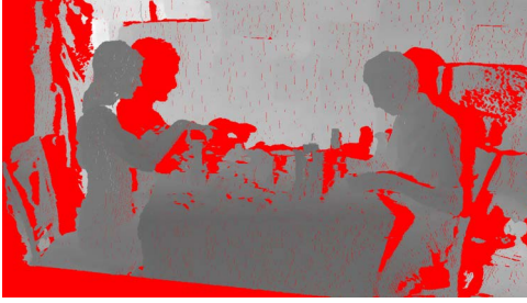
(a) Forward warping without filtering. Red areas denote unknown pixels. Note that there are thin regions with red values as well as thin regions with background pixels that are visible through what should be a solid foreground object, due to the discretization of the source pixels' coordinates.
