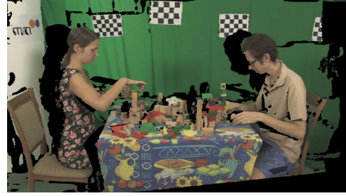
Fig. 2. Pixels from a known camera have been warped on the view of a virtual camera. As the camera movement was to the left, parts of the background that were not visible to the original camera are now disoccluded.
