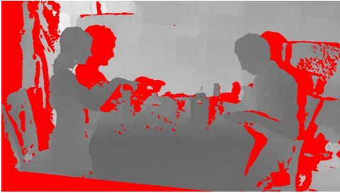
(b) The proposed depth map filter successfully fills depth pixels that should be known or corrects depth pixels that are likely to be wrong.
